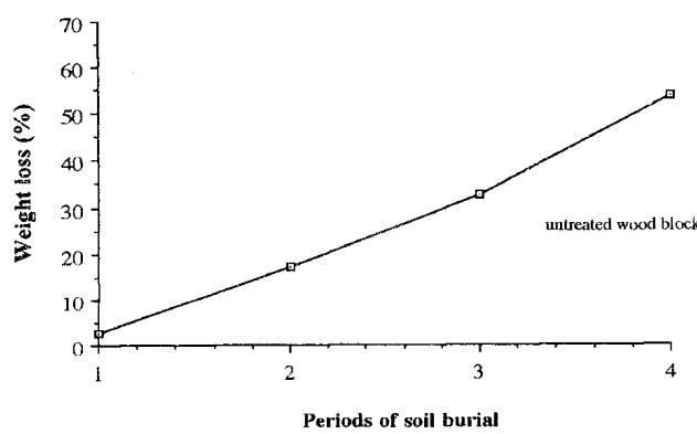
**Figure 3. Mean percent weight loss of untreated wood blocks through soil burial**
